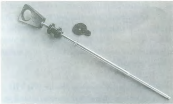
Fig. VIIIa. Double ring loading mechanism using a rubber washer (separate)
