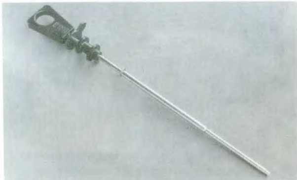
Fig. VIIIb. Double ring loading mechanism with rubber washer in situ.
